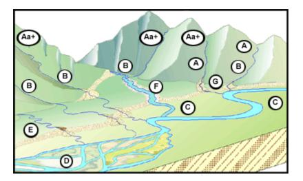
The figure above shows how different Level I stream types tend to appear in different parts of the landscape. With proper training, Level I classification can be delineated on common information sources such as topographic maps and aerial photographs.
