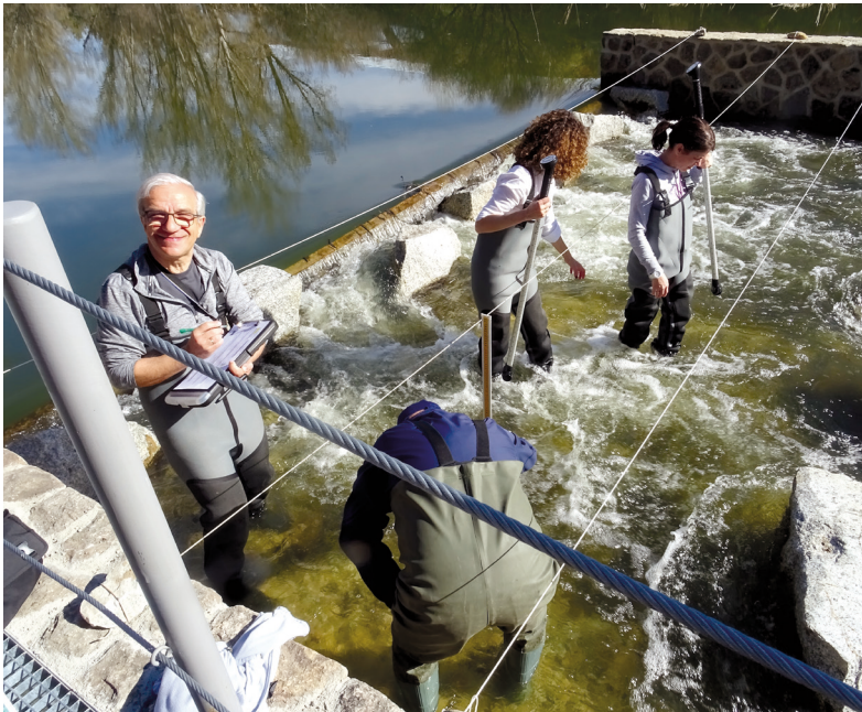
FIGURE 40 Monitoring campaign for the estimation of depths and velocities
