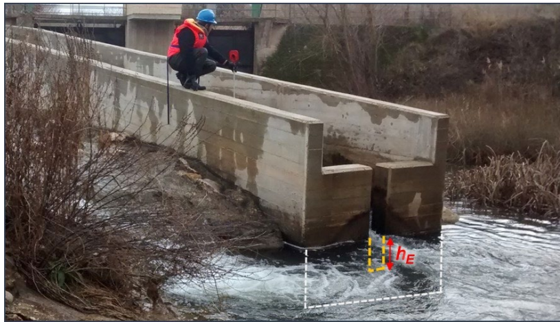
Figure 12. Diagram of depth at the entrance, where the edge of the entrance opening is shown in yellow and the variable is shown in red.
